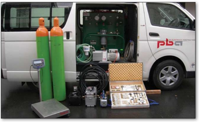
PBA's Enervac GRU-6 SF<sub>6</sub> Gas Cart and SF<sub>6</sub> accessories are easily transported in our vans
